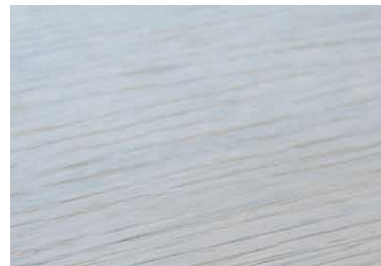
Laminate produced with impress modifier. No heat tearing.
