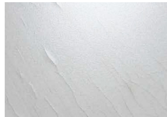
Laminate produced without a resin modifier. Product can suffer from heat tearing.
