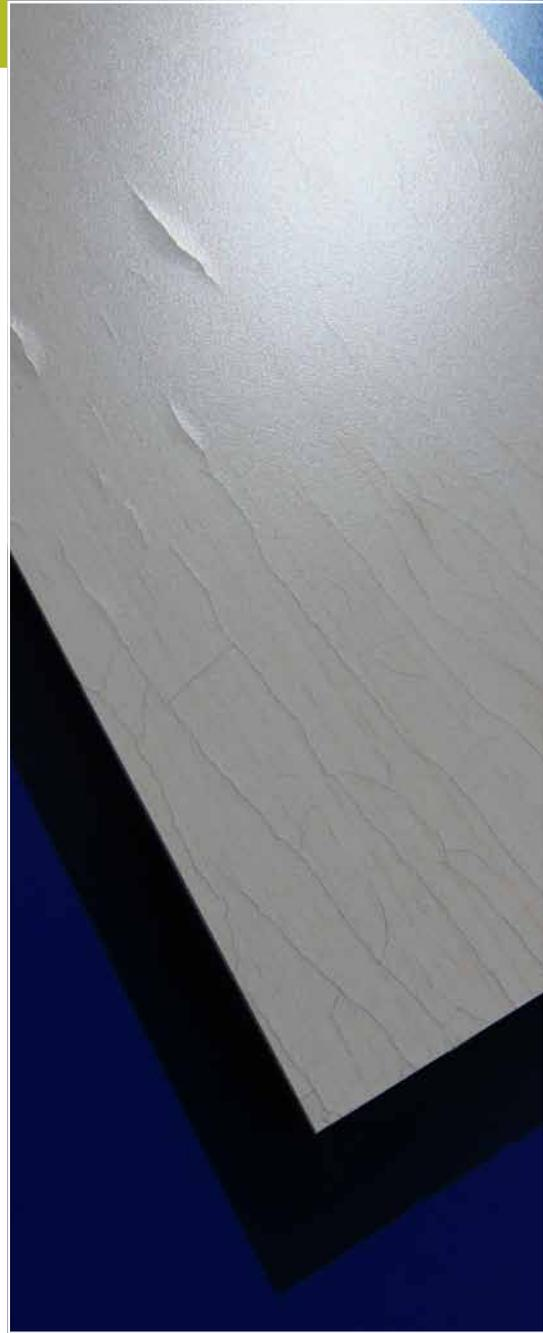
Laminate produced without a resin modifier.
